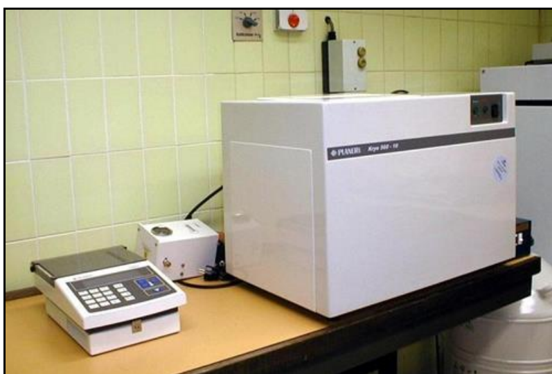
Figure 4. Device for controlled-rate freezing of isolated cells
